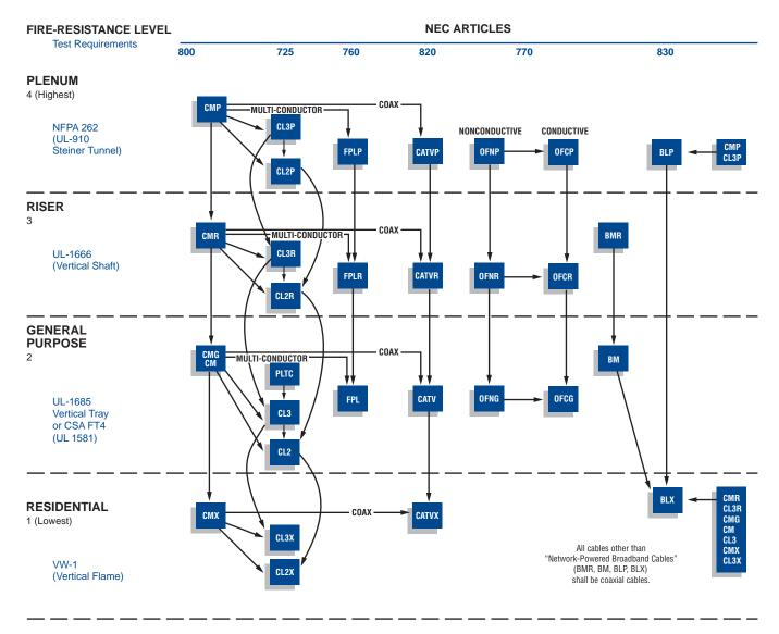
Cables indicated can be substituted.
